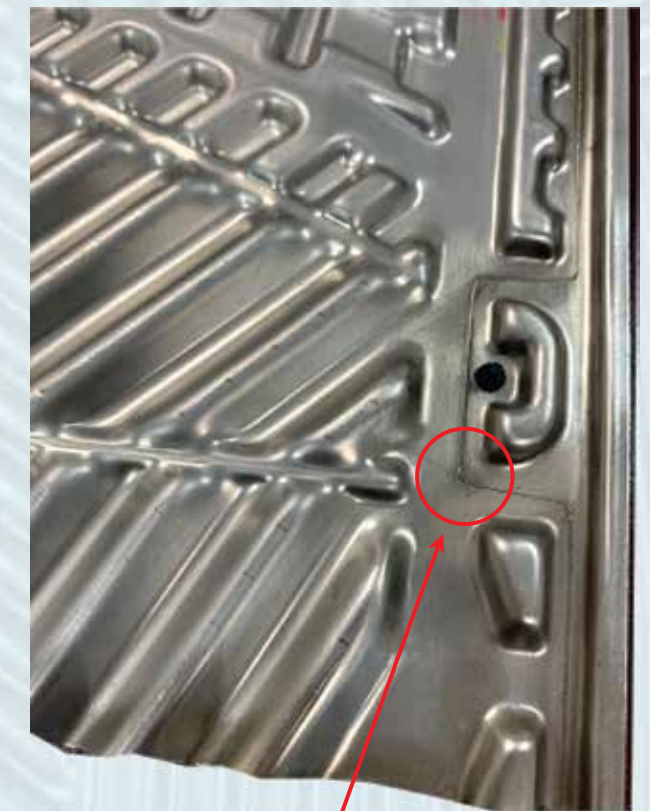
Two plates Laser Welded
